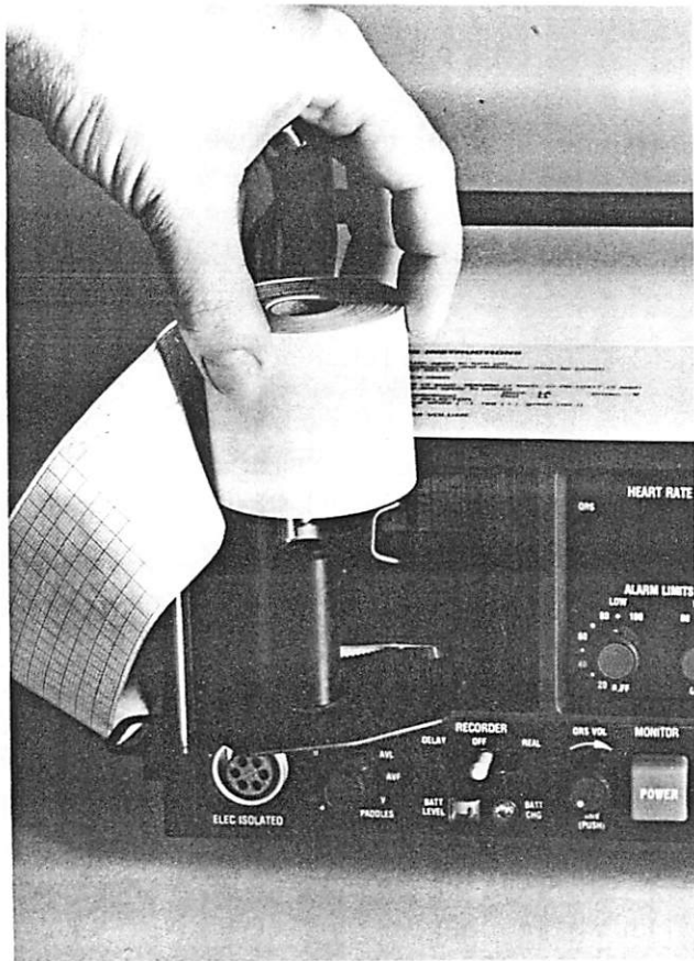
Figure 2-5 Recorder Paper Replacement
