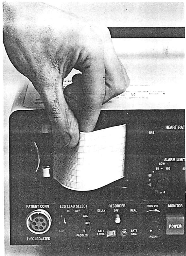
Figure 2-5 Recorder Paper Replacement
